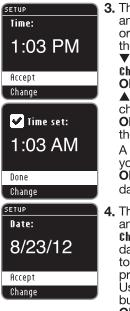
3. The time will appear and you can ficcept or Change. To change the time, use the ▼ button to select Change and press the OK button. Use the ▲ or ▼ buttons to change and press the OK button to move to the next item.
