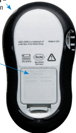
Battery – Insert with (+) symbol facing up.
